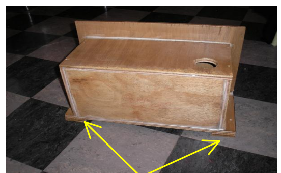
Bottom of the box, showing the battens that offset the back from the wall
