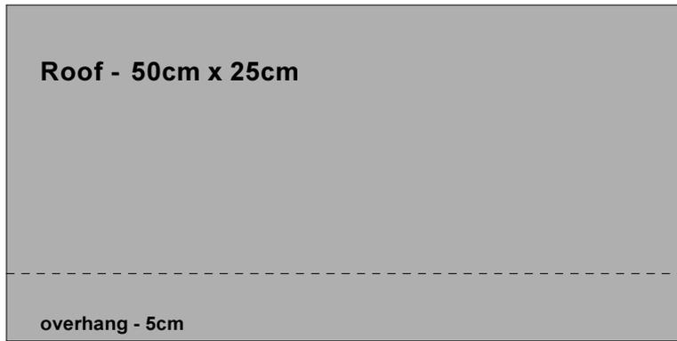
Make up from 12mm to 15mm thick weatherproof exterior quality or marine ply.
